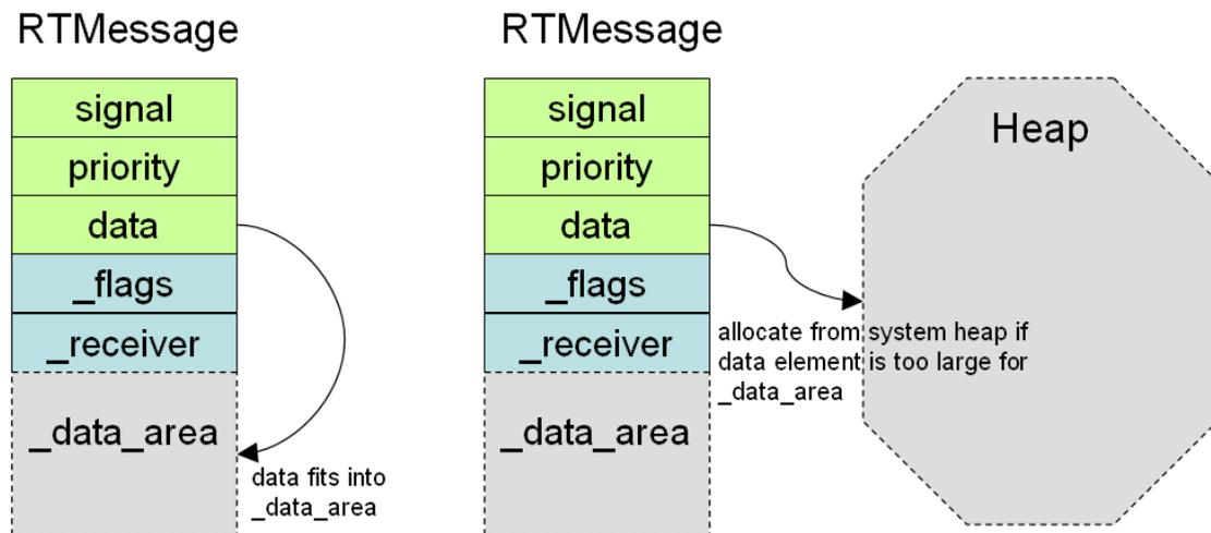
Each `RTController` object has a pool of allocated `RTMessage` objects that are free of data and that are used when a new message should be sent. This pool is called the "free list":
