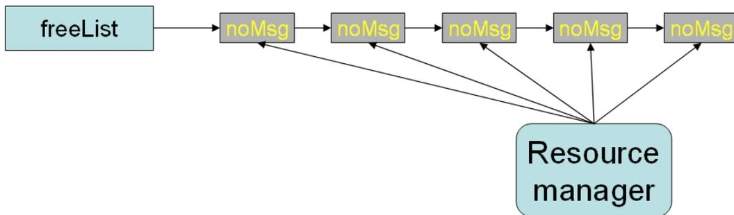
When a thread needs to send a message, the resource manager takes the next free message object in the `freeList` of the corresponding `RTController` object and returns it to the controller that will fill in all message information and send the message. If there is no free message in the list, a new bunch of messages are allocated in the system heap with the call to the function
