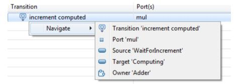
Here the memory-based search command has returned a transition in the model. In addition to the transition itself you can navigate to the port referenced by one of its triggers, the source and target states as well as the owner capsule to which the transition belongs.
