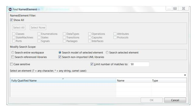
For now let's ignore the various settings which are provided by this dialog, and jump directly to the text field in the middle of the dialog. Here you can type the name of the element you are looking for. As soon as you stop typing for a moment, a search will start in the background. A message is shown in the status bar while the search runs:
