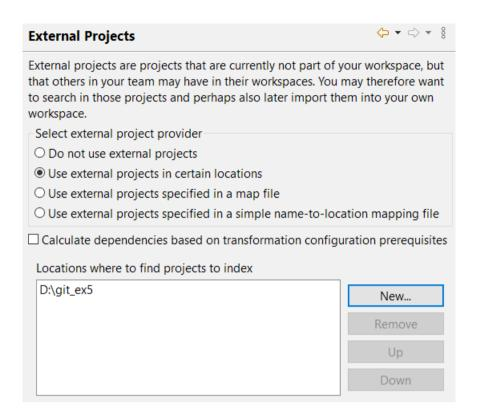
External projects can be specified either as a list of locations in the file systems (i.e. folders), or a map file can be used for specifying the external projects. The map file is a text file where each external project is specified on a separate line using the syntax
