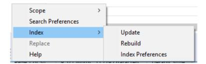
Choose *Index - Update* to update the index, and *Index - Rebuild* to completely rebuild the index from scratch.
